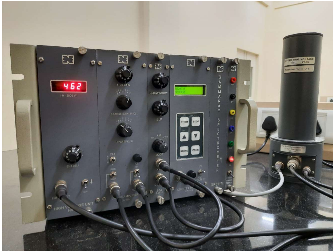
Figure 6: (Left) Gamma-ray spectrometer system GR611M and (Right) Detector assembly (NaI + PMT + preamplifier) set up in the laboratory.
